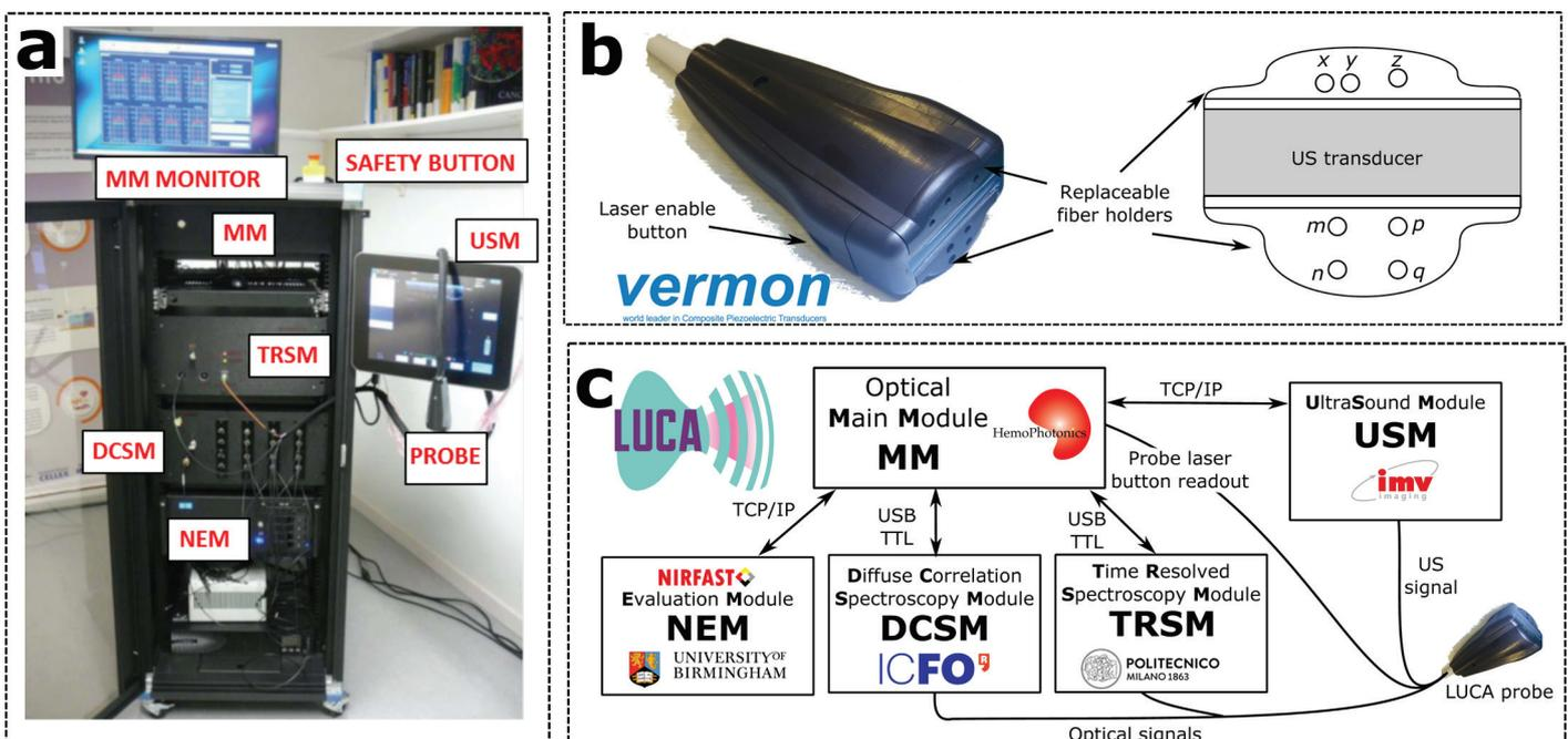
Description: Photo of the LUCA device with all the components (a), the head of the probe (b) used for scanning the thyroid, and the specific component developed by each of the consortium members.
